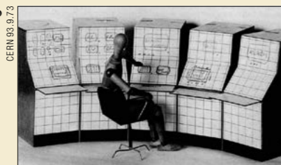
Not the result of a life test on a machine operator but simply a bit of ergonomics while working out the best layout of the consoles for the SPS control room.
