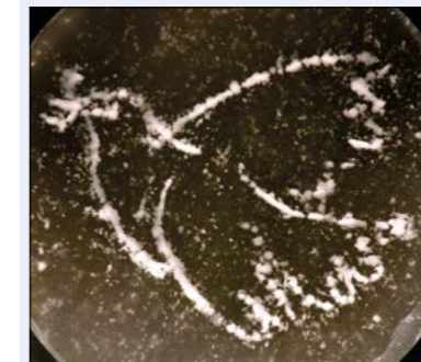
Ultrasonic waves were used to push a collection of microparticles into the shape of Picasso's peace dove. (Image credit: K Melde/MPI for Intelligent Systems.)
