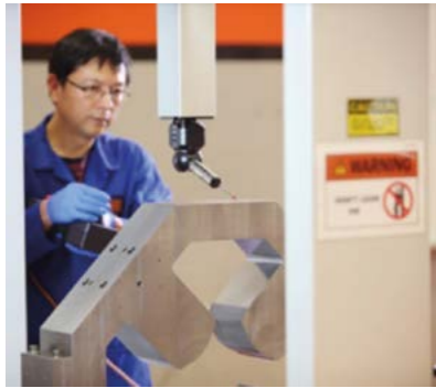
Mobile "Roamer" CMM used to confirm dimensions are within tolerance on a quadrupole magnet.
